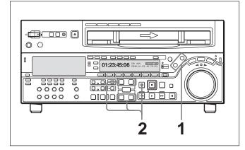
**1** Press the RECORDER button or PLAYER button to select the VTR on which you wish to operate.
